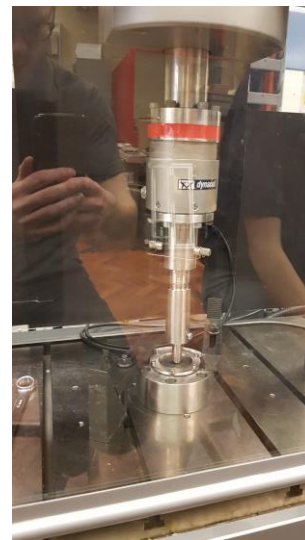
Figure 3: Dynamic stress testing of sensor from 600-6000 N, at 2 Hz.
