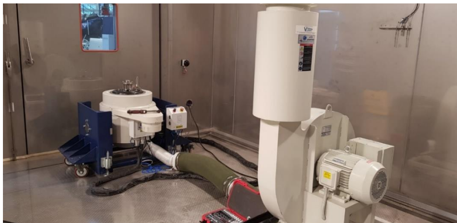
Figure 1: Vibration testing of Ionix sensors. The sensors are able to operate normally (launching and receiving ultrasound) at up to 40g acceleration, from 100 to 4,000 Hz.
