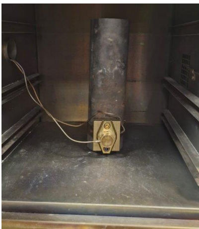
Figure 1: Wall thickness monitoring through temperature cycling, demonstrating long-term durability
