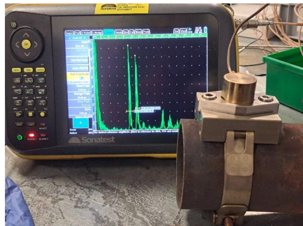
Figure 2: Lead-free HotSense™ probe connected to a 3" pipe with a deployment system
