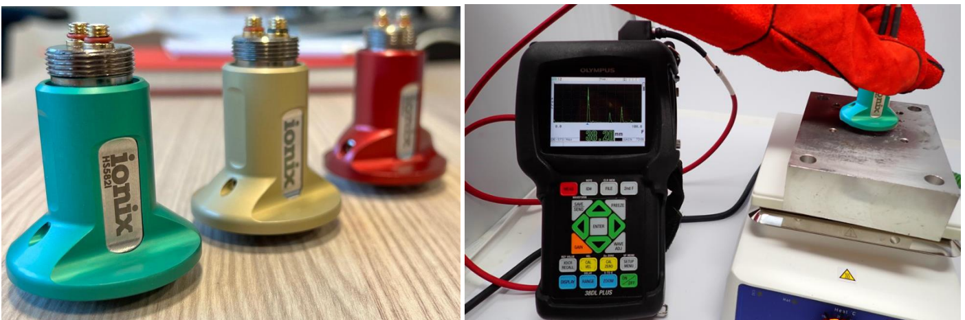
Figure 1: (left) a photograph of HotSense HS582i probes assembled with lead-free materials. (right) ultrasonic testing being completed with an off-the-shelf gauge, with continuous contact to an aluminium block at 300 °C.
