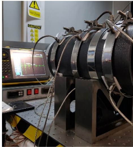
Image 1 – Low profile transducer platform using HPC attached to a pipe section operating at 350 °C
