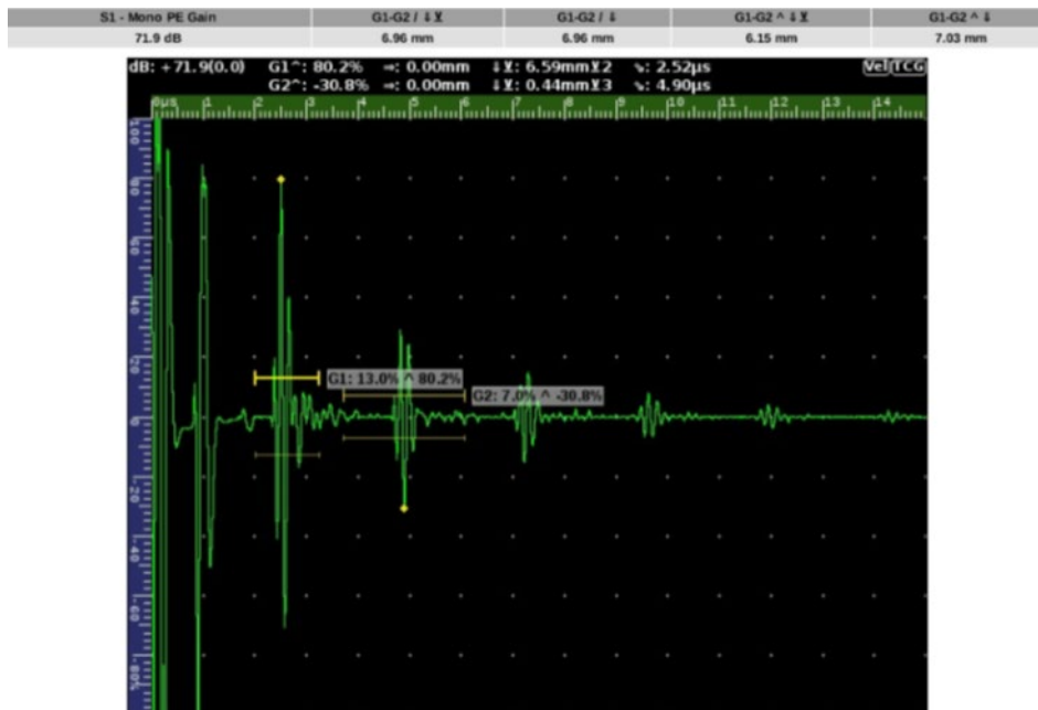
Image 3 – A-scan from a HPC transducer at 350 °C
